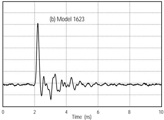
A 0.15-ps pulse at 1.06  $\mu\text{m}$  was used to test the photodetectors, and the output was measured using a 12-GHz oscilloscope.
